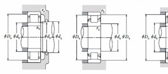
High quality cylindrical roller bearing with machined brass cage from the leading manufacturer TIMKEN. Featuring the TIMKEN EMA design. A premium land-riding cage, unique internal geometries, enhanced surface finishes and a compact design. All this adds up to longer life, improved uptime and reduced maintenance costs.
